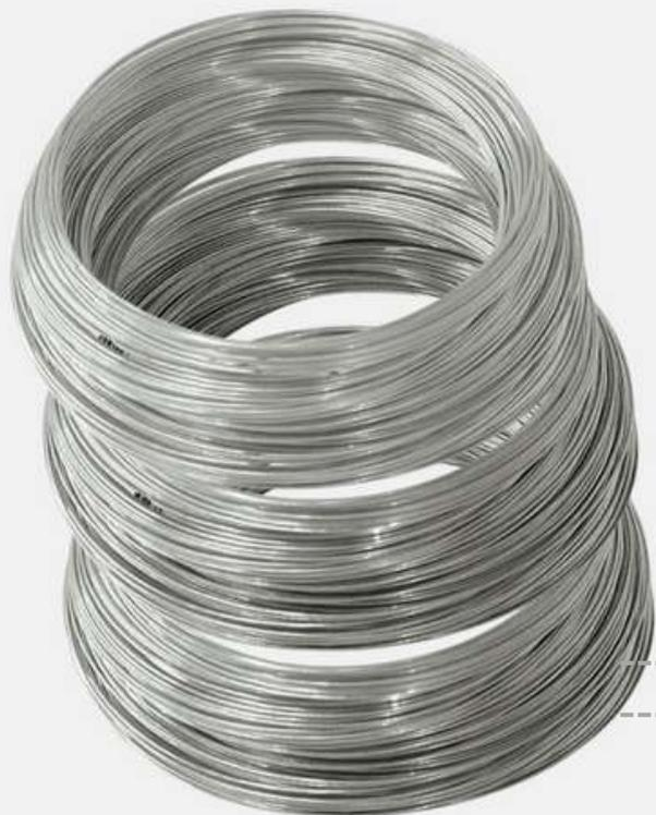
Galvanized BWG wire is a low carbon steel wire, this wire material is widely used for connecting bones to other bones, BWG wire or better known as zinc wire or slippery wire is made through the process of drawing, pickling, rust removal, strengthening and cooling, and covered with a galvanic process. The series between bones are in the form of column bones, beam bones, practical columns, sloof or other bones. So that this wire becomes a support for a series of elements that are ready to be cast.
