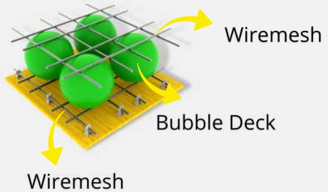
BubbleDeck is a patented integration technique for connecting air, steel and concrete in a two-way structural slab. The hollow plastic ball is inserted into the plate and held in place with reinforcing steel. This concept is based on the fact that the area between columns of solid slabs has a limited structural effect beyond weight gain.
